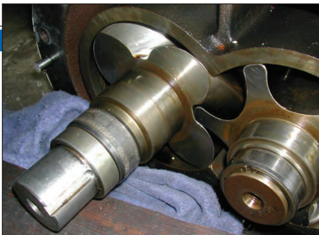
FIGURE 1. In an oil-injected, twin-screw compressor, the lubricating oil is injected into the gas stream to absorb the heat of compression and act as lubricant and sealant. This enables a much higher pressure ratio in a single stage and provides significant protection against corrosive gases. In multi-stage machines, inter-cooling is usually not required
