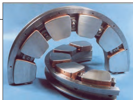
FIGURE 3. Tilting-pad bearings are commonly used for high-speed rotating machines. Each bearing consists of a series of pads. Because oil is basically incompressible, pressure builds within the oil film, which provides a means for the oil film to transfer the load
